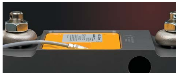
Small details improve durability. The EDXtreme features a recessed connector and embedded antenna to help prevent damage from snags that commonly disable other instruments.
